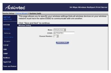
**6.** In next Wizard screen, the wireless network security settings are configured. From the "Encryption Mode" text box, select "Disabled," "WEP," or "WPA-shared key," depending on the type of encryption the wireless network is using. If the network is not using encryption, select Disabled, click **Save & Next**, and go to step 7. If WEP or WPA-shared key is selected, continue to the next page.
